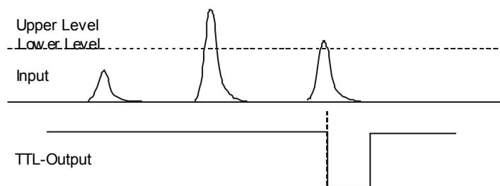
Each SCA 6030 is equipped with two independent SCA channels. For the measurement of Radon e.g. the measurement of the Radon-progeny plated out on the detector surface (Po-218 and Po-214), the channels are adjusted to enable the determination of fast changes in the Radon concentration as well as long term measurements:
