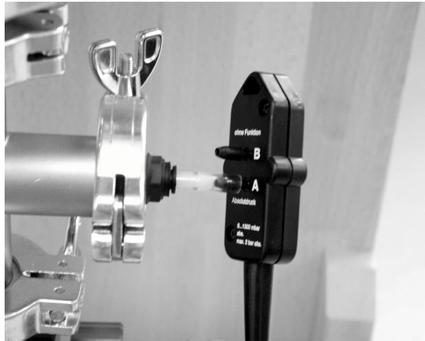
Correct connection of pressure gauge to the T-junction
