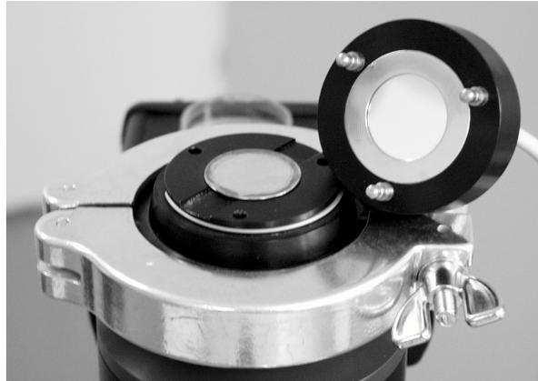
Screen with replaced detector head
