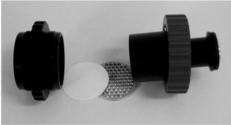
Backup filter stage (left to right): Filter holder, filter, prop, exhaust to pump
