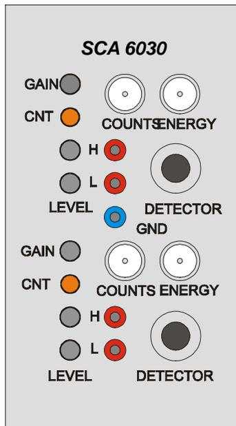
The SCA 6030 supports when used together with the calibration drum, the 400 mm<sup>2</sup> Si-detector that is fixed in the diffusion bell and placed within the calibration drum.
