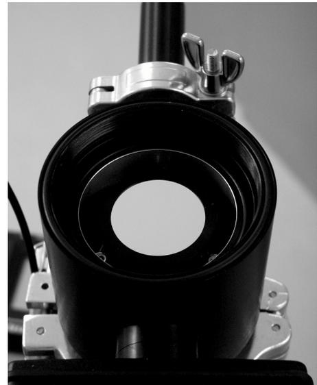
Impactor stage with removed red inlet tube. On the left can see the orifice with screwed on tool, the right picture enables an insight on the foil which covers the detector.
