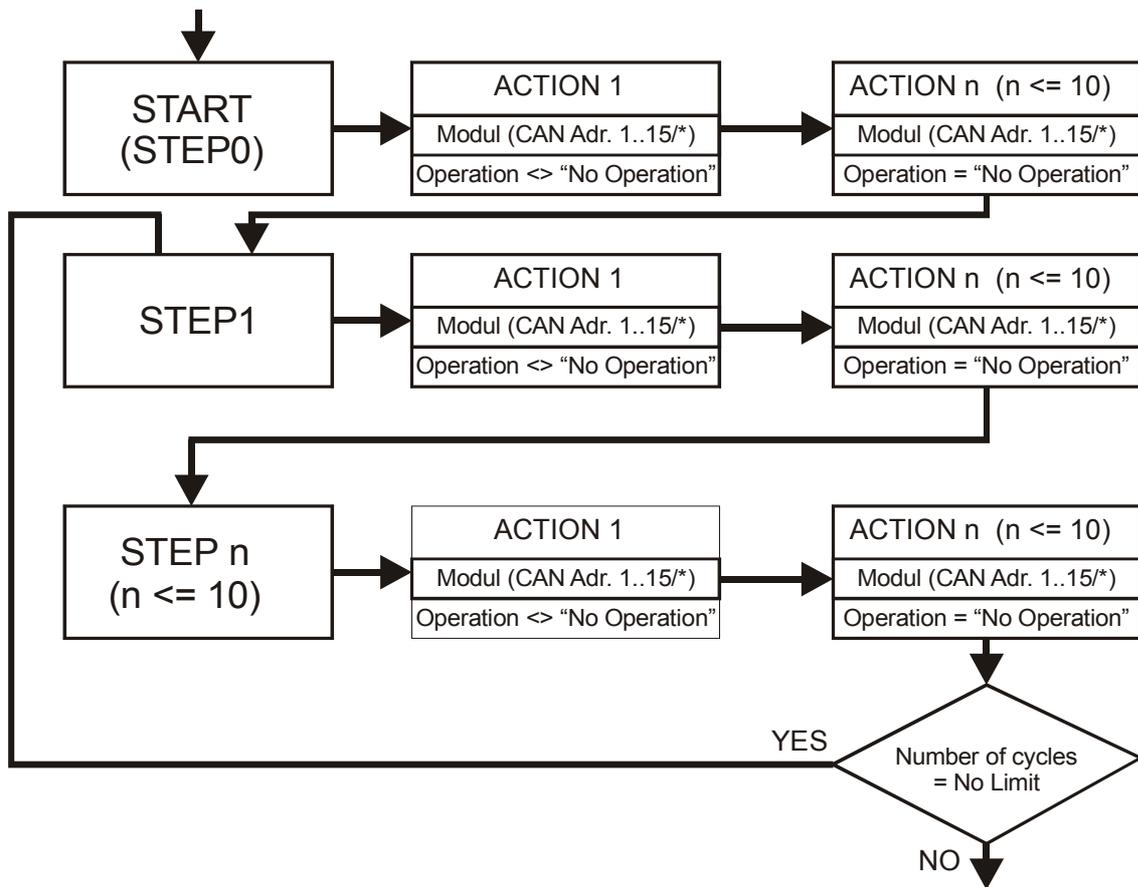
Each measurement cycle consist of up to 10 different steps with different time intervals. Each step consist of up to 10 actions that will be executed at the end of the step.
